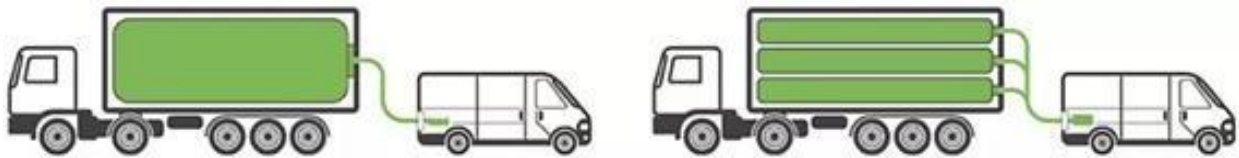
Figure 13. This diagram depicts decent technology (left) versus cascade technology (right). NanoSUN uses cascade for hydrogen refueling
