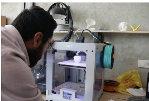
Figure 40. 3D printing with recycled building materials
