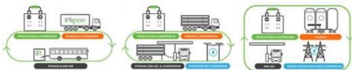
Figure 14. This diagram illustrates the advantages of NanoSUN's mobile Pioneer Hydrogen Refuelling Station (HRS) solutions (furthest left) in comparison to fixed HRS solutions (center and right)
